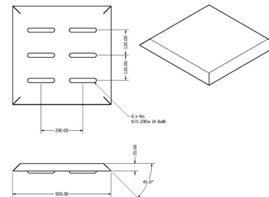
Six bulbs are mounted in the positions shown above in Figure 37: lamp and reflector arrangement. Each bulb must have a rated output of 200W and be of clear glass type. All bulbs should be replaced after a maximum of 150 hours of operation.
