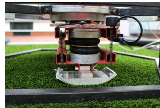
Start the rotation of the test foot. Allow the test foot to make five complete revolutions at a speed of  $40 \pm 1\text{rpm}$ , sampling at a minimum frequency of 40Hz.
