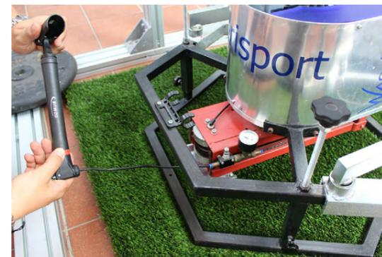
**Figure 35:** test foot in position having the load applied
