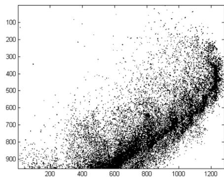
The frames are then transformed into two-colour black-and-white images (RGB 000 – red, green, blue colour model) and cropped to ensure that none of the yarn and undisturbed infill is included in the image. The percentage of black-to-white pixels in the image is calculated. The highest “splash percentage” is then recorded as the test result.
