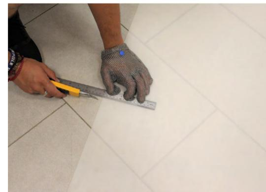
Figure 20: silicon skins cut and ready to be cleaned
