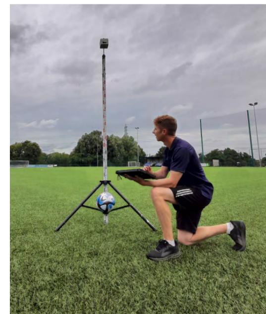
NB: To limit the influence of the valve, it should preferentially be positioned at the top of the ball when the ball is attached.
