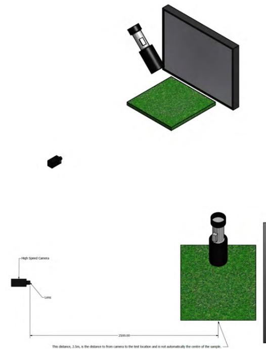
The camera must be angled with the lens to the horizontal at  $5 \pm 1^\circ$  and the height off the ground adjusted so that the cross-sectional profile of the sample is visible with the visible splash window as large as possible.
