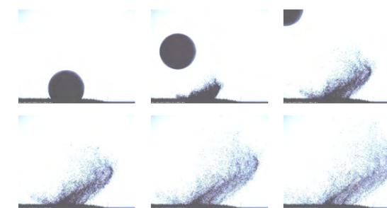
The ball is projected onto the sample from the cannon and the impact on the surface is recorded using a high-speed camera. The full interaction from the point at which the ball impacts the surface is captured.
