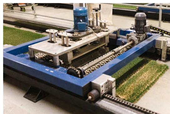
**23 PROCEDURE FOR SIMULATED MECHANICAL WEAR ON ARTIFICIAL TURF - LISPORT XL (FIFA TEST METHOD 2024-13)**
