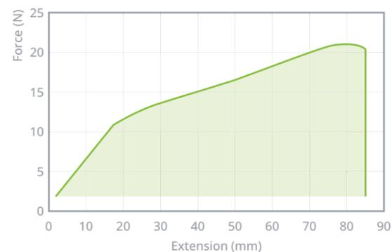
The area under the stress-strain curve represents the energy absorbed by the material before failure, allowing for a comparison between ductile and brittle materials. In the context of synthetic turf, a ductile yarn is considered to be more resilient than a brittle yarn based on their respective behaviours and energy absorption capabilities.
