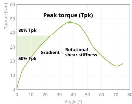
Report the mean rotational shear stiffness to the nearest 0.01Nm/°, e.g. 0.92Nm/°. The uncertainty of measurement in rotational shear stiffness is  $\pm 0.05$  Nm/°.
