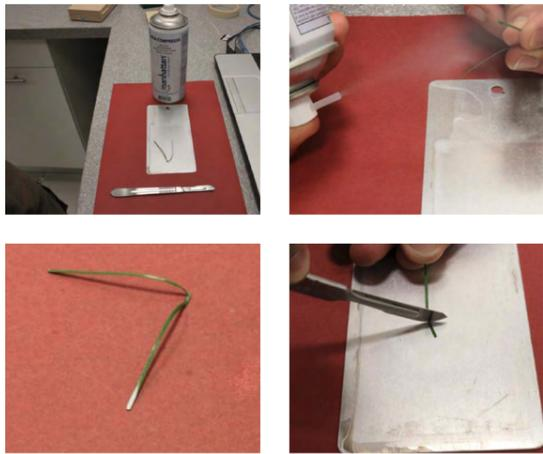
Using a support, holding the cut end in a vertical position perpendicular to the microscope, verify that the cut is clean, and if necessary, depending on the colour of the fibre, use an insert of a different coloured background to maximise the definition of the image.
