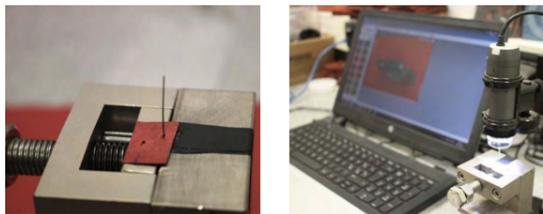
Adjust the magnification of the microscope in the range of 200-250x and focus on the cross-sectional cut plane of the fibre. After making sure that they are in focus, take the picture.
