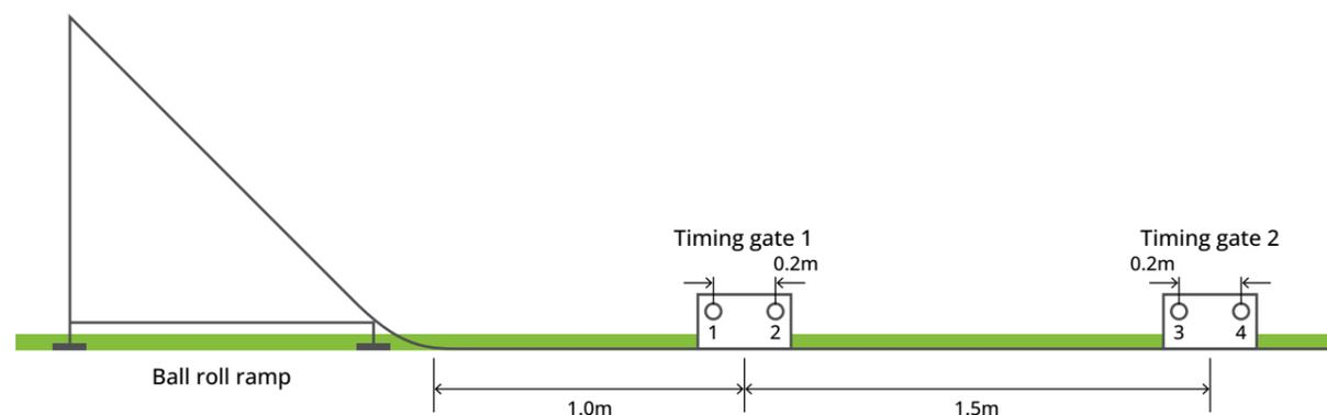
Four release heights should be selected on the ramp from which to release the ball, as shown in Figure 7: ball release heights. Release height 1 should be the lowest height selected on the ball ramp. This should be adjusted to ensure that the ball stops between 0.1m and 0.25m past the second timing gate. The final release height is the highest and should be the same as a standard ball roll, namely  $1.0 \pm 0.01$  m.
