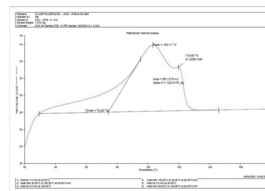
The peak is clearly broader in Figure 51: DSC curve representing melting behaviour of a fibre with a blend of polymers, and there is a shoulder at approximately around 120°C.
