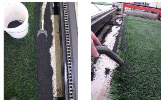
Carefully redistribute the infill material collected over the conditioned area; ensure a homogeneous distribution using an appropriate application device as shown below in Figure 44: redistribution of dispersed infill.
