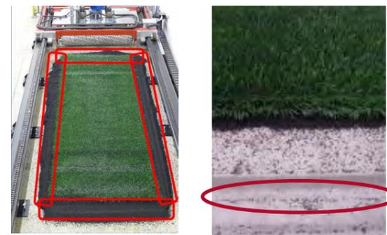
**Figure 43:** examples of infill collection
