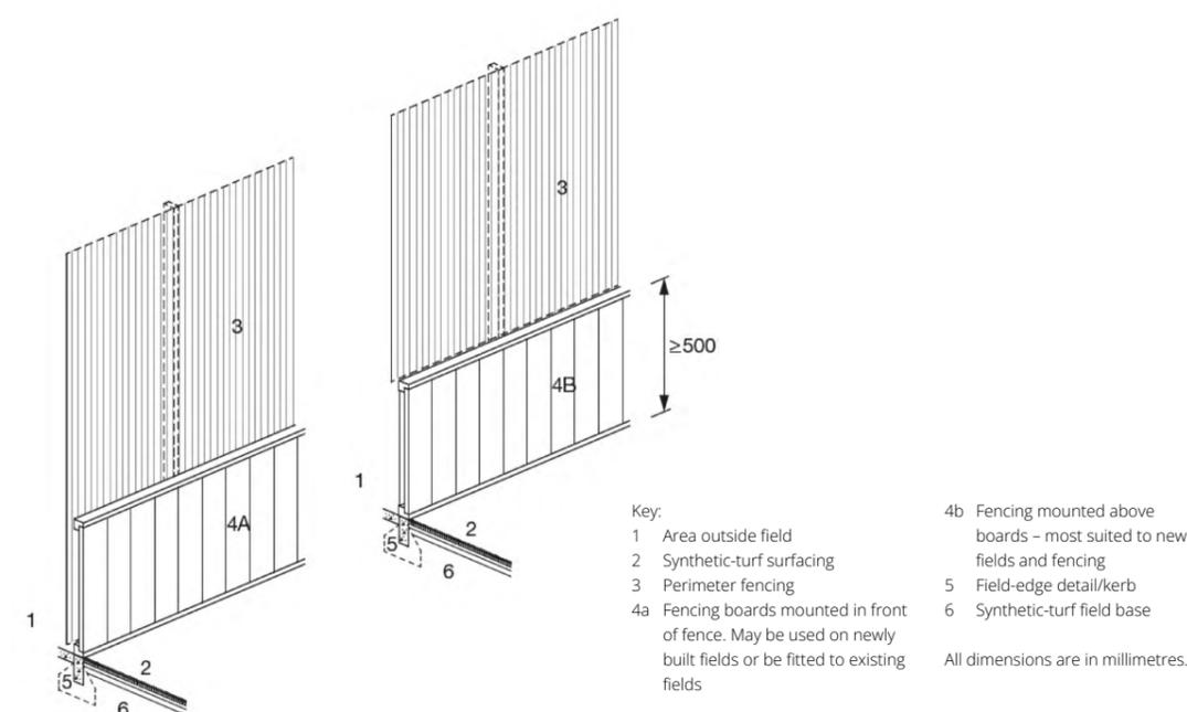
**Figure 65:** raised edging options and paved zone to separate synthetic-turf surface from perimeter boundary
