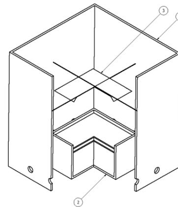
**22.2.1 Apparatus enclosure marked as "1" in Figure 36: sectional schematic of apparatus for measuring heat (temperature increase) above**
