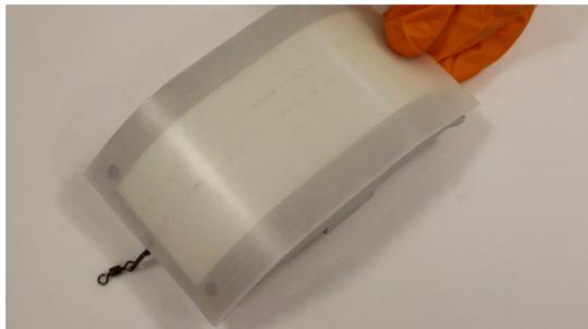
Punch holes on the silicon skin to apply the fixing screws using a die cutter or a suitable tool.
