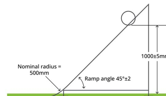
**Figure 4a:** additional ball roll length measurement procedure
