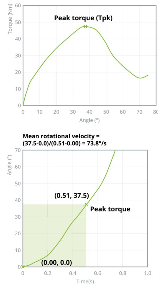
Find the peak torque and the time at which it occurs. The peak torque represents the rotational resistance.
