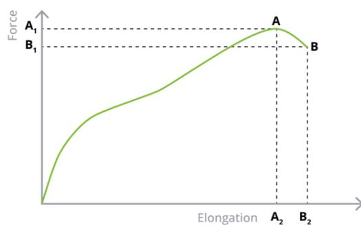
Yarn brittleness reflects the yarn's ability to absorb energy, which is determined by the area beneath the force-extension curve generated during testing. The impact of artificial weathering on yarn samples, leading to yarn degradation, is assessed through changes in this energy absorption capacity.
