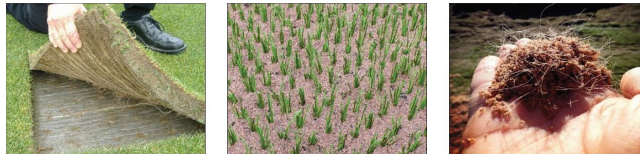
Fig. 5. Types of turf reinforcement system. From left to right: carpet, stitched and fibre
