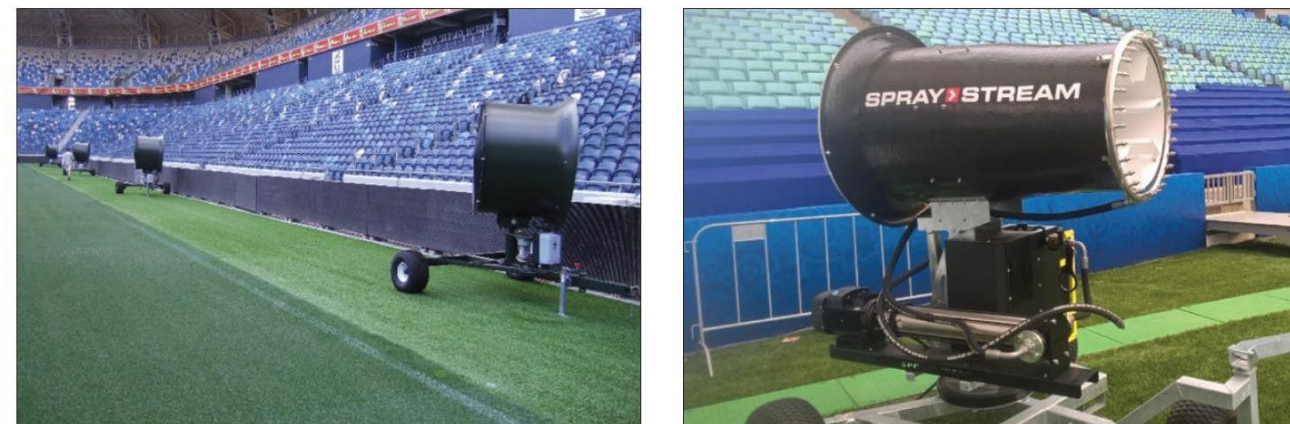
Fig. 11. Examples of pitch side ventilation and cooling fans used to manage turf health
