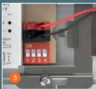
DIP switch for easy power steps setting.
